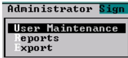
The light gray bar positioned on the 'Lookup' selection when the menu is first displayed is a selector bar. Functions may be selected from the menu by moving the selector bar with the arrow keys and then pressing the Enter key to select the function. (When a sub-menu is displayed, the selector bar is black because the sub-menu is displayed in a light gray.) There is an expanded description of the currently highlighted function displayed on the line below the current user's ID Number and name.
